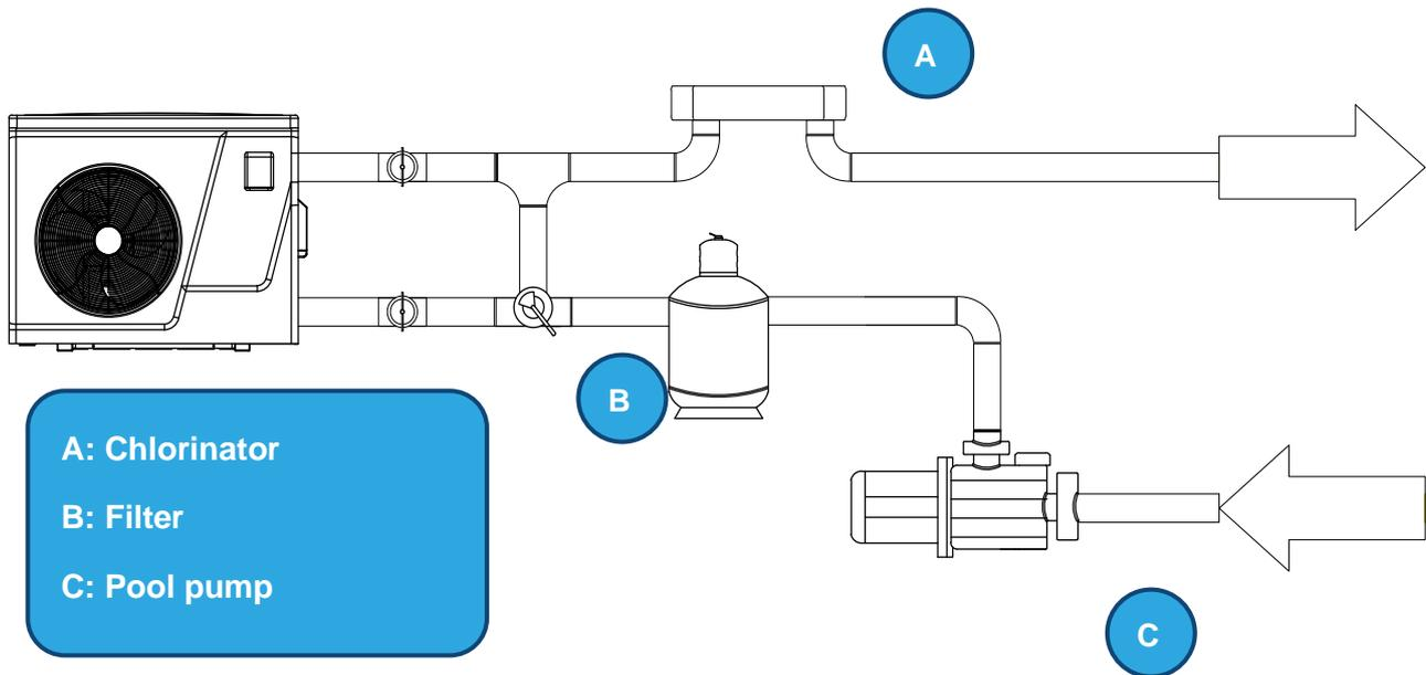
1. Chlorinator controller initiates the filtration pump.
