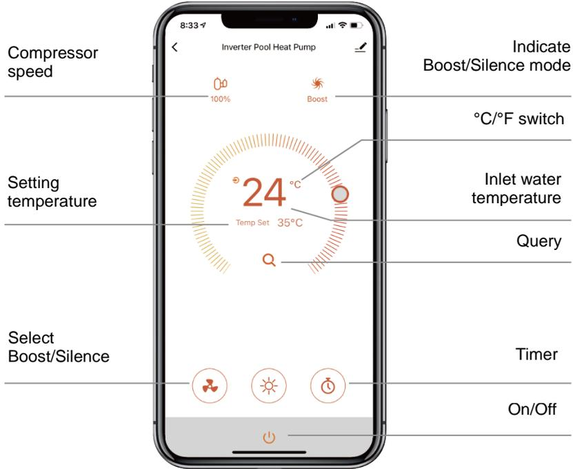
2. For heat pump with Heating & Cooling function:
