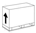
b. Do not lift with the water unions(The titanium heat exchanger inside the heat pump may be damaged)
