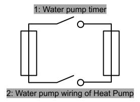
Note: The installer should connect 1 parallel with 2 (as above picture). To start the water pump, condition 1 or 2 is connected. To stop the water pump, both 1 and 2 should be disconnected.
